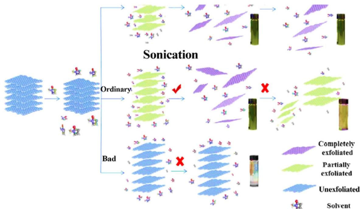
Fig. 9 A schematic illustration of the liquid-phase exfoliation method.<sup>191</sup>
