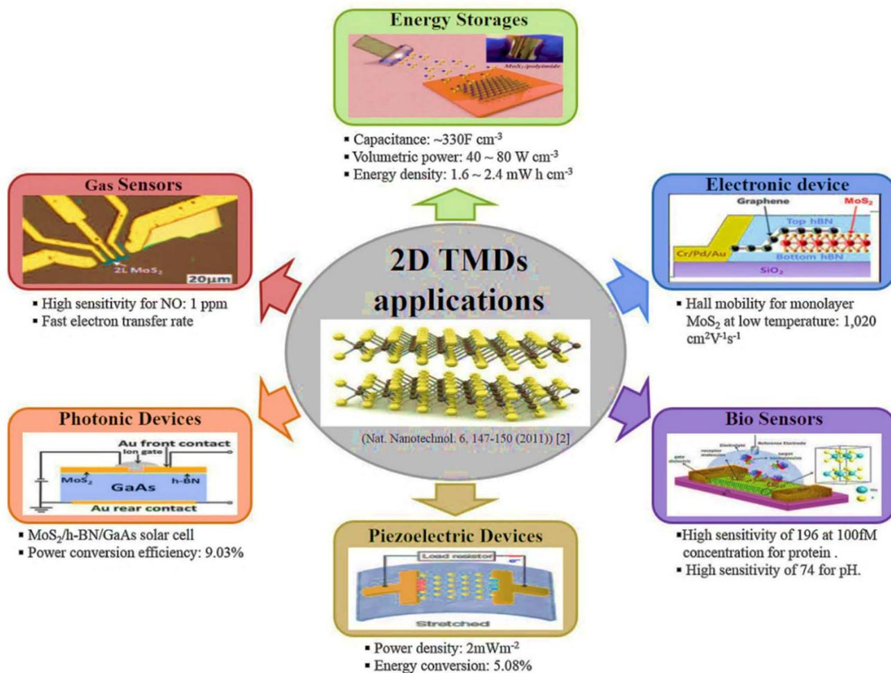
Fig. 12 Electronic, optoelectronic and energy devices based on 2D TMDs. Reproduced from ref. 210 with permission from Elsevier, copyright 2017.
