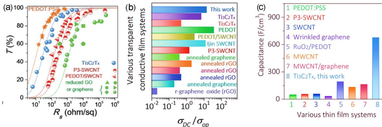
Fig. 24 Optoelectronic properties of  $\text{Ti}_3\text{C}_2\text{T}_x$  films: (a) the transmittance ( $T$ ) at  $550 \text{ nm}$  as a function of sheet resistance  $R_s$  and (b) comparison of  $\text{Ti}_3\text{C}_2\text{T}_x$  with other transparent thin films. (c) Comparison of  $\sigma_{DC}/\sigma_{op}$  in  $\text{Ti}_3\text{C}_2\text{T}_x$  films to various other transparent capacitive electrodes (TCEs). Reproduced from ref. 379 with permission from John Wiley and Sons, copyright 2017.
