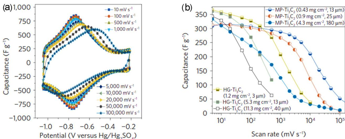
Fig. 23 (a) Measurement of CV for a 90 nm thick  $\text{Ti}_3\text{C}_2\text{T}_x$  MXene at scan speeds ranging from 10 to 100 000  $\text{mV s}^{-1}$ . (b) The gravimetric rate performance of MXene film preparation procedures and mass loading dependence. Reproduced from ref. 373 with permission from Springer Nature, copyright 2017.
