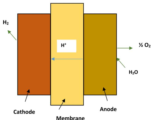
Fig. 5 PEM electrolysis cell.
