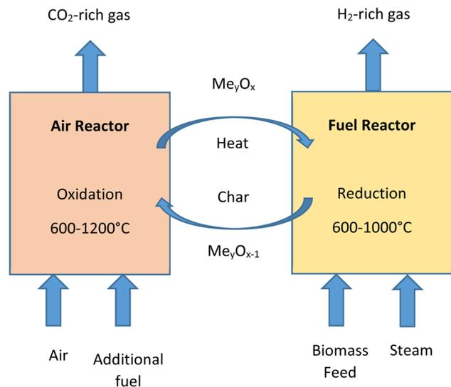
Fig. 10 A schematic of chemical looping gasification.
