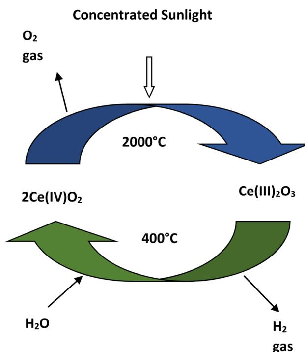
Fig. 7 Two-step cerium oxide water splitting cycle.
