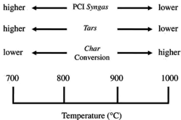
Fig. 8 [Fig. 2 influence of temperature process on the syngas characteristics.] Adapted from Molino, A., Chianese, S., & Musmarra, D., Biomass gasification technology: the state of the art overview. *Journal of Energy Chemistry*, 2016, 25(1), 10–25, DOI: 10.1055/s-0035-1560215.
