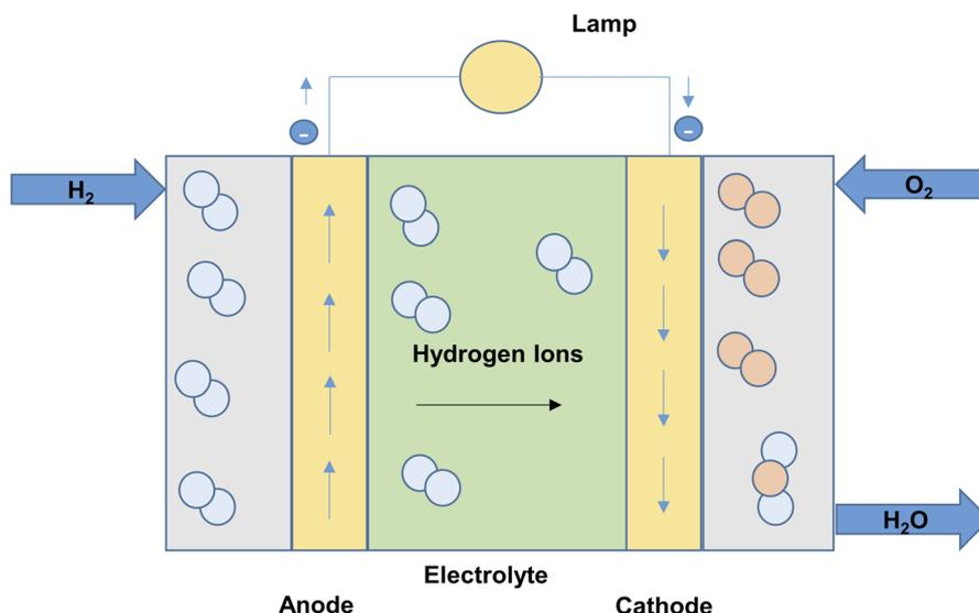
Fig. 13 A schematic of PAFC.
