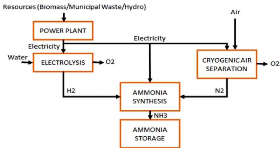
Fig. 12 [Fig. 9 ammonia production via hydrogen electrolysis and H–B process.] Adapted from Valera-Medina, A., Xiao, H., Owen-Jones, M., David, W. I., & Bowen, P. J., Ammonia for power. *Progress in Energy and combustion science*, 2018, **69**, 63–102, DOI: 10.1016/j.pecs.2018.07.001.
