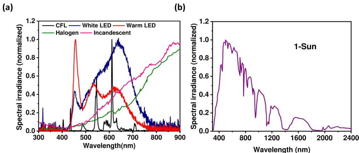
Fig. 1 (a) Irradiance spectra of different indoor light sources;<sup>16</sup> (b) solar spectra (AM1.5G).<sup>16</sup>
