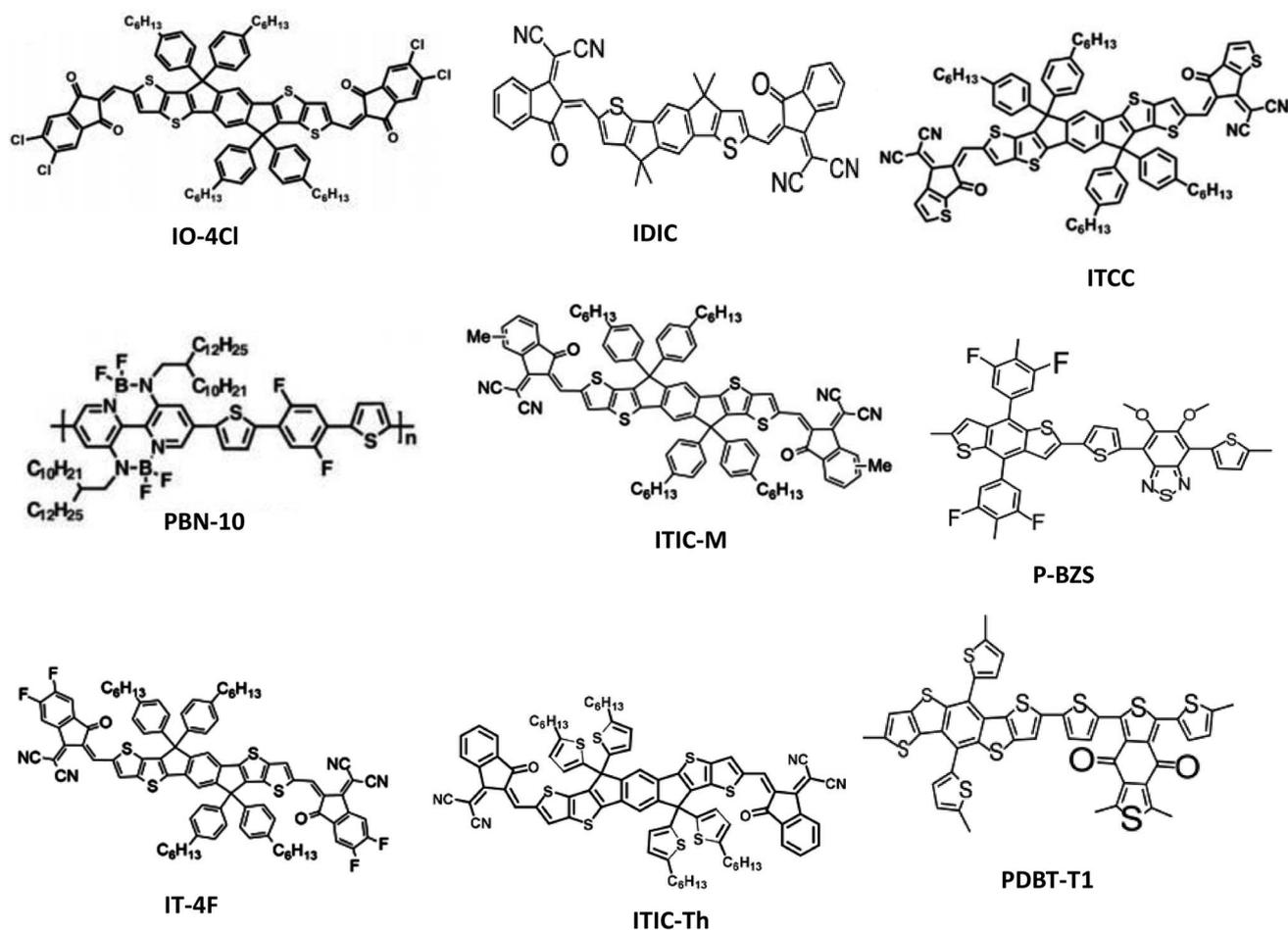
Fig. 5 The chemical structures of different non-fullerene-acceptor materials utilized in indoor OPVs.
