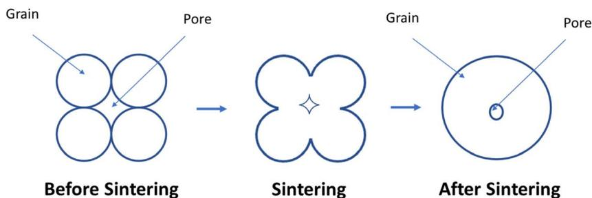
Fig. 10 How pore size reduces during sintering process.
