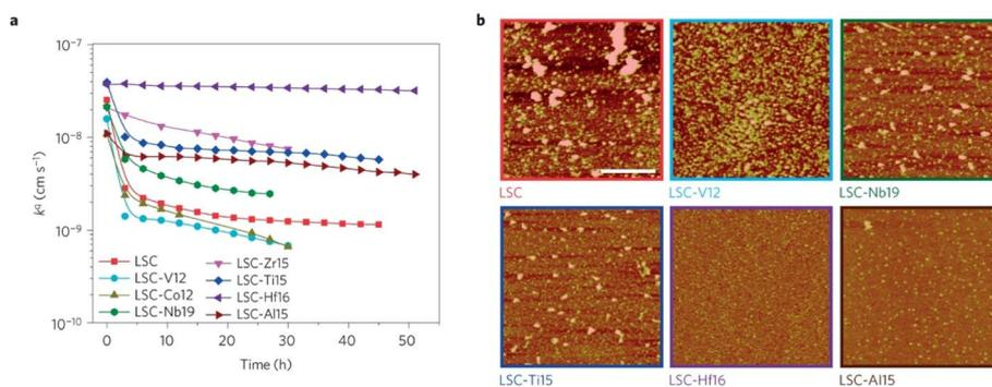
Fig. 21 (a) Oxygen surface exchange coefficient,  $k^q$ , quantified from electrochemical impedance spectroscopy measurements over time at 530 °C in air, for the LSC and LSC-Me films. (b) Atomic force microscopy images of the LSC, LSC-V12, LSC-Nb19, LSC-Ti15, LSC-Hf. (Reproduced with permission from ref. 56 Copyright 2016 Nature.)
