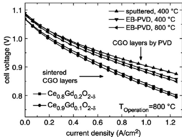
Fig. 32  $I$ - $V$  curves of cell with sintered and physical-vapor-deposited GDC buffer layers run at 800 °C. (Reproduced with permission from ref. 84 Copyright 2007 Elsevier.)
