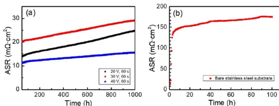
Fig. 24 (a) *In situ* monitored ASR values for spinel coated samples at 700 °C for up to 1000 h and (b) ASR of the uncoated 460FC stainless steel substrate, measured under a current load of  $10 \text{ mA cm}^{-2}$ . (Reproduced with permission from ref. 122 Copyright 2022 Elsevier.)
