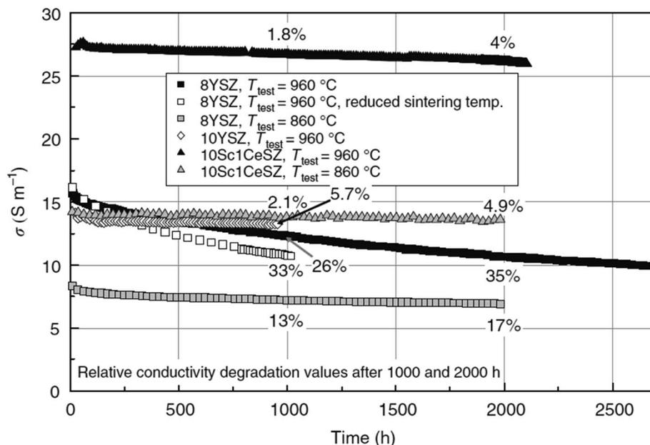
Fig. 1 Degradation of conductivity of ceramic materials over a span of 2500 h of continuous testing. (Reproduced with permission from ref. 20 Copyright 2009 Elsevier.)
