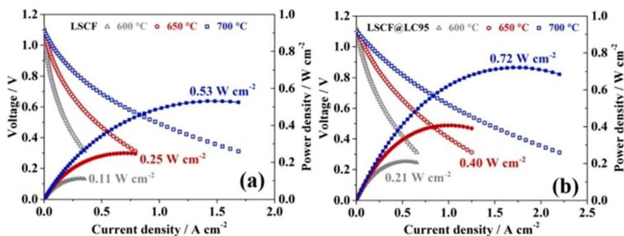
Fig. 18 Performance and durability of single cells:  $I$ – $V$ – $P$  curves of single cells with (a) LSCF and (b) LSCF@LC95 cathode at intermediate temperature range. (Reproduced with permission from ref. 113 Copyright 2022 Elsevier.)
