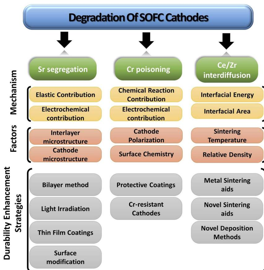
Fig. 4 Simplified overview of degradation of SOFC cathodes.
