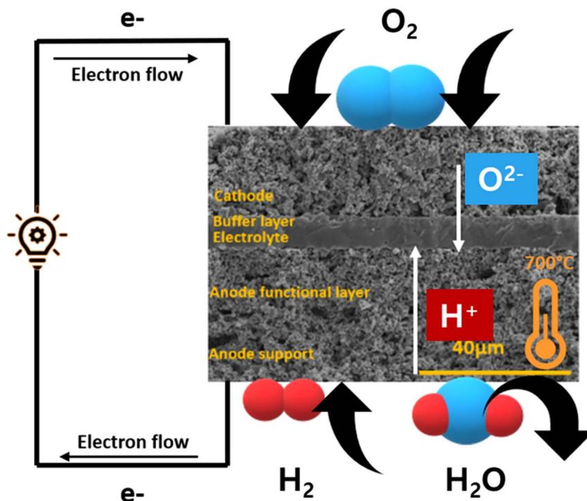
Fig. 5 Schematics of a typical  $O^{2-}$  conducting SOFC.
