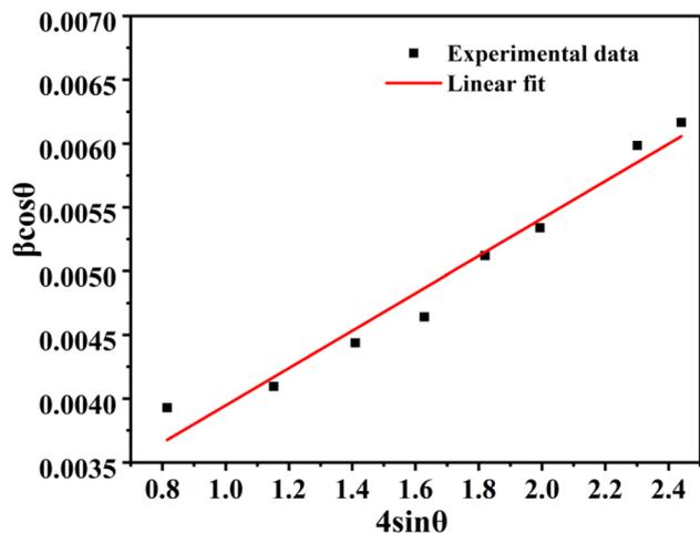
Fig. 5 Williamson–Hall (W–H) plot of  $\text{La}_{1-x}\text{Ce}_x\text{AlO}_3/\text{MgO}$  ( $x = 0.7$  mol%).
