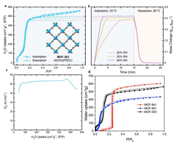
Fig. 36 Water adsorption properties of MOF-303. (a) Water adsorption isotherm at 30 °C. (b) Water vapor adsorption  $\theta$  desorption behavior. (c) Isosteric heat of adsorption ( $Q_{st}$ ) for MOF-303. Reproduced from ref. 116 with permission from ACS central science. (d) Water adsorption isotherm of MOF-303 compared to other hydrophilic MOFs. Reproduced from ref. 101 with permission from ACS central science.
