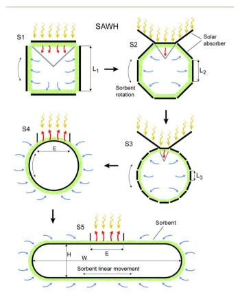
Fig. 38 Schematic of semi-active systems. Reproduced from ref. 156 with permission from Energy & Environmental Science.
