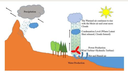
Fig. 12 The process of a SCPP with water vapor condensation on the sea surface. Reproduced from ref. 62 with permission from Energy Conversion and Management.
