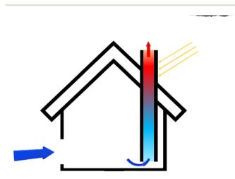
Fig. 11 Schematic of solar chimney
