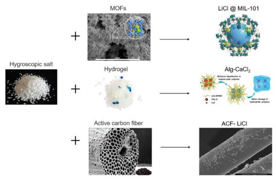
Fig. 26 Composite desiccants. Reproduced from ref. 83 with permission from Solar Energy Materials and Solar Cells
