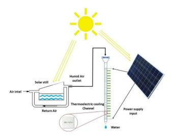
Fig. 9 Schematic of TEC-based distillation system.
