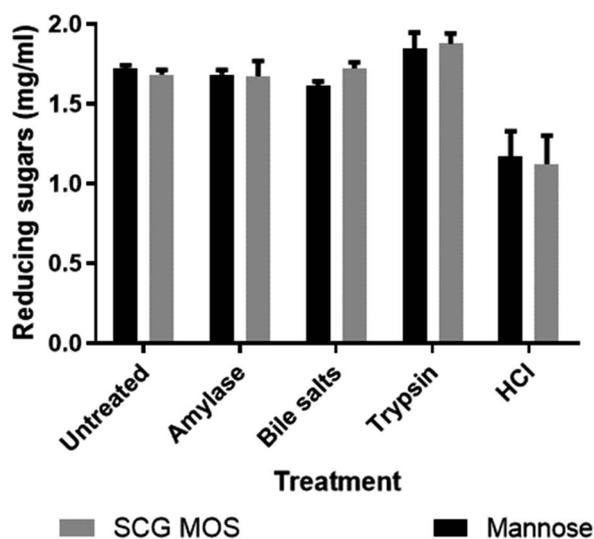
Fig. 4 Effect of bile salts,  $\alpha$ -amylase, trypsin and hydrochloric acid (pH 1.5) on SCG MOS. Values are represented as means  $\pm$  standard deviations,  $n = 4$ . An equal amount mannose ( $1.7 \text{ mg mL}^{-1}$ ) was treated the same as the MOS to test their recovery post treatment.
