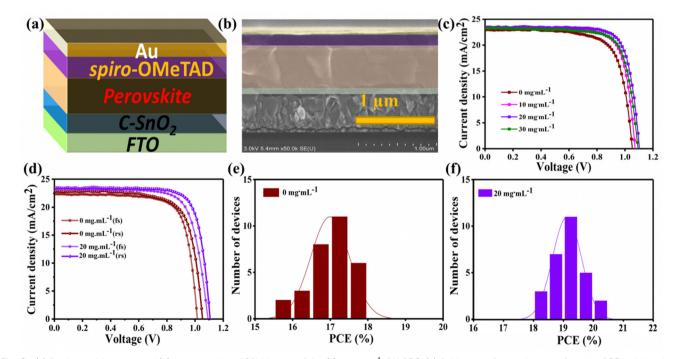
Fig. 6 (a) Device architecture and (b) cross-sectional SEM image of the 20 mg mL<sup>-1</sup>-FAI PSC. (c) J–V curves for the best-performing PSCs with various FAI concentrations. (d) J-V curves of control and 20 mg mL<sup>-1</sup>-FAI treated PSCs with reverse and forward scans. Distribution PCE of (e) 0 mg mL<sup>-1</sup> and (f) 20 mg mL<sup>-1</sup>-FAI treated devices. There are 30 and 28 devices of the statistical distribution of PCEs for control and 20 mg mL<sup>-1</sup>-FAI PSCs.
