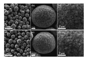
Fig. 1 (a-c) SEM images of a pristine LiNi<sub>0.6</sub>Co<sub>0.2</sub>Mn<sub>0.2</sub>O<sub>2</sub> (NCM622) sample. (d-f) SEM images of coated NCM622 prepared from a ballmilling method with Nb<sub>2</sub>O<sub>5</sub> (0.5 mol%). Reproduced with permission from ref. 76. Copyright 2021, Elsevier.
