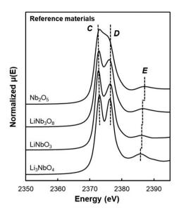
Fig. 3 XAS of the Nb L<sub>3</sub>-edge of reference materials with Nb<sup>5+</sup> oxidation state. Dotted lines C and D correspond to LiNbO<sub>3</sub> peak position, while dotted line E is peak position of each reference material. Reproduced with permission from ref. 57. Copyright 2023, American Chemical Society.
