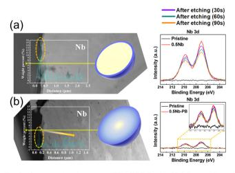
Fig. 2 Cross-sectional scanning TEM (STEM) with EDS line profiles of Nb across the yellow line for LiNi<sub>0.82</sub>Co<sub>0.12</sub>Mn<sub>0.06</sub>O<sub>2</sub>. Shown to the right is the corresponding material's Nb 3d XP spectra with different etch times. Panel (a) refers to a coating methodology of introducing Nb, while panel (b) refers to a route of including Nb with the precursor reagents. Adapted from ref. 87. Copyright 2021, American Chemical Society.
