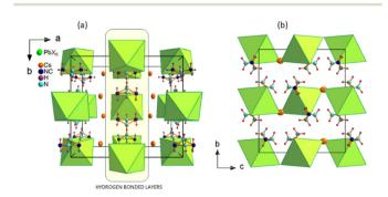
Fig. 1 The crystal structures of  $Cs_2MHy_2PbX_6$  and  $MHy^+$  are disordered. (a) Discrete (0D) Pb  $(Br/I)_6$  units interact through HBs with MHy<sup>+</sup> cations forming HB layers perpendicular to the *a* direction, coulombic interactions between caesium ions and Pb(Br/I)<sub>6</sub> units stabilize the structure perpendicular to the layers. (b) The view along the *a* direction.
