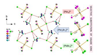
Fig. 2 The N-H...Br HB network in Cs<sub>2</sub>MHy<sub>2</sub>Pb(Br/I)<sub>6</sub>. In each Pb(Br/I)<sub>6</sub> there are two sites for halogen ions interacting with middle-chain NH<sub>2</sub> groups. In Cs<sub>2</sub>MHy<sub>2</sub>PbI<sub>3</sub>Br<sub>3</sub> they are preferentially occupied by Br<sup>-</sup>.
