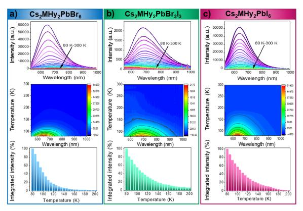
Fig. 6 Temperature-dependent emission spectra recorded from 80 to 300 K, the PL intensity contour map, and the integrated emission intensity at various temperatures of (a) Cs<sub>2</sub>MHy<sub>2</sub>PbBr<sub>6</sub>, (b) Cs<sub>2</sub>MHy<sub>2</sub>PbBr<sub>3</sub>I<sub>3</sub>, and (c) Cs<sub>2</sub>MHy<sub>2</sub>PbI<sub>6</sub>, respectively.
