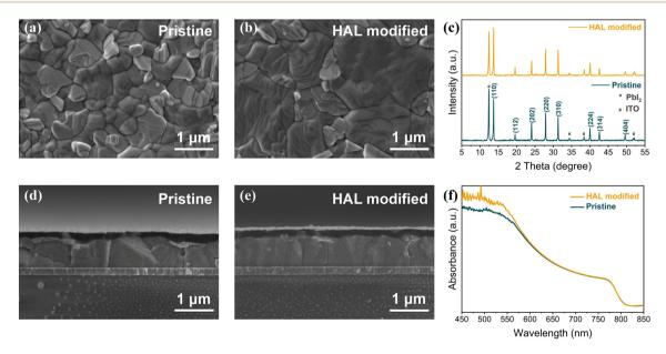
Fig. 2 Top-view SEM images of PVK films with (a) pristine and (b) HAL-modified SnO<sub>2</sub> films. (c) XRD patterns and (f) UV-Vis absorption spectra of PVK films with different SnO<sub>2</sub> films. Cross-sectional SEM images of PSC devices with (d) pristine and (e) HAL-modified SnO<sub>2</sub> films.
