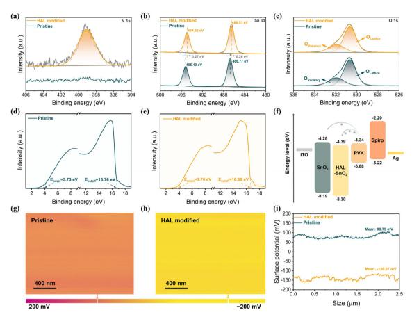
Fig. 1 (a) N 1s, (b) Sn 3d, and (c) O 1s XPS spectra of different SnO<sub>2</sub> films. UPS spectra of (d) SnO<sub>2</sub> and (e) HAL-modified SnO<sub>2</sub> films. (f) Energy band diagram of the materials employed in PSCs. KPFM images of (g) SnO2 and (h) HAL-modified SnO2 films. (i) Surface potential of different SnO2 films.
