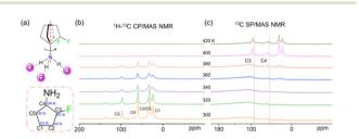
Fig. 3 (a) The rotating motion mode and C atoms naming and corresponding chemical shift of polar rotor TFCA. (b) $^{1}H-^{13}C$  CP/MAS NMR spectra of 1 around 300-420 K. (c) <sup>13</sup>C SP/MAS NMR spectra of 1 at the range of 300-420 K.
