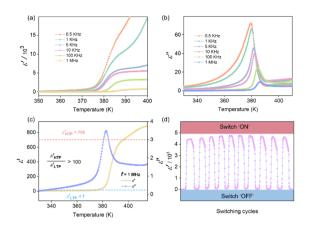
Fig. 4 The dielectric anomaly measurement of polycrystalline samples of 1. (a)  $\varepsilon'$  at different frequencies upon heating. (b)  $\varepsilon''$  at different frequencies upon heating. (c)  $\varepsilon'$  and  $\varepsilon''$  at 1 MHz. (d) After 10 switching cycles at a frequency of 25 kHz, the value of the dielectric constant shows a sensitive switchable with no decrease.
