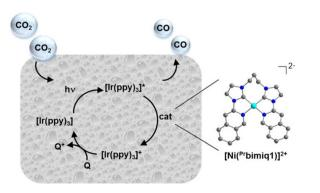
Fig. 1 Photocatalytic CO<sub>2</sub> reduction process by the [Ni(Prbimig1)]<sup>2+</sup> complex. Reprinted with permission from ref. 26. Copyright 2013 American Chemical Society.
