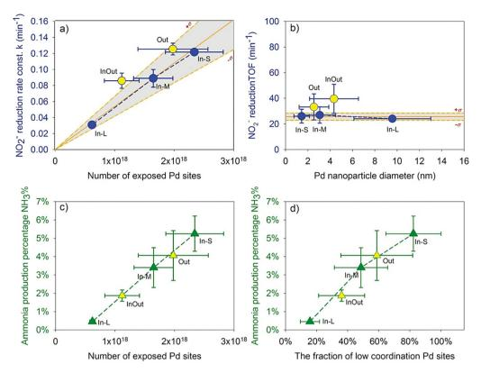
Fig. 8 (a) First-order rate constant (k) versus the number of exposed Pd sites. (b) TOFs versus Pd NP diameters. (c) Ammonia production percentage (NH<sub>3</sub>%) versus the number of exposed Pd sites. (d) Ammonia production percentage (NH<sub>3</sub>%) versus the fraction of low-coordination Pd sites.<sup>3</sup> Copyright 2021, American Chemical Society.
