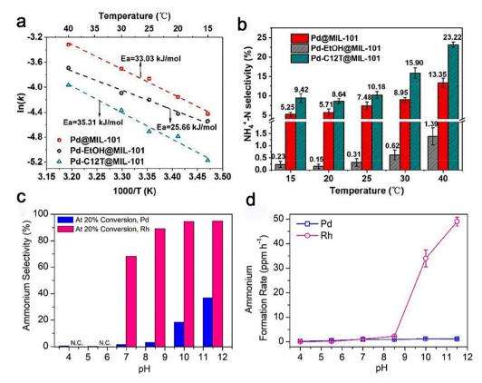
Fig. 7 (a) Experimental estimation of nitrite reduction activation energies ( $E_a$ ) on different Pd surfaces. (b) Effects of the reaction temperature on ammonia selectivity on various Pd surfaces. 38 Copyright 2018, the Royal Society of Chemistry. (c and d) Effects of varying pH values on the selectivity of ammonia and the ammonia production rates on Pd and Rh.<sup>87</sup> Copyright 2019, American Chemical Society.
