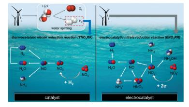
Fig. 13 Simplified reaction mechanism of the thermal nitrate reduction reaction (TNO<sub>3</sub>RR) and the electrocatalytic nitrate reduction reaction (ENO<sub>3</sub>RR). 146 Copyright 2018, the Royal Society of Chemistry.
