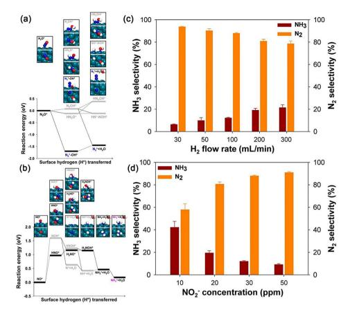
Fig. 9 (a) Energy diagram of the hydrogenation pathway of NO\* on a Pd(111) surface. (b) Energy diagram of the reduction of N₂O\* on Pd(111). Insets show the reaction intermediates considered for calculations. Green, blue, red, and white spheres represent Pd, N, O, and H atoms, respectively. (c and d) Experimentally measured N2 and NH3 selectivity of nitrite reduction at various (c) H2 flow rates and (d) NO2- concentrations. 15 Copyright 2014, American Chemical Society.
