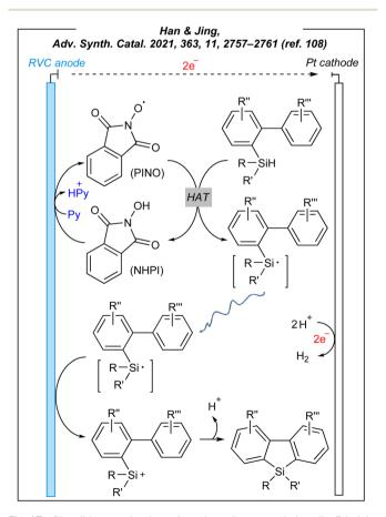
Fig. 13 Plausible mechanism for the electrocatalytic sila-Friedel-Craftss reaction.
