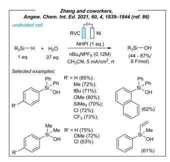
Fig. 7 Silanol-oriented hydrolysis of hydrosilanes under electrochemical conditions.
