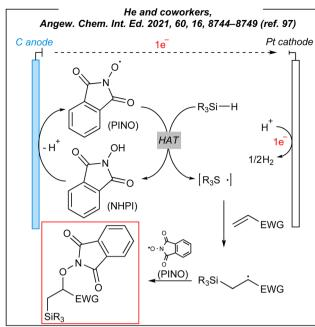
Fig. 11 Plausible mechanism for the 1,2-silylfunctionalization.
