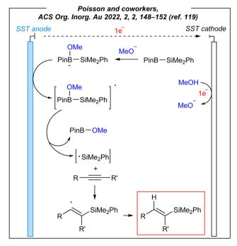
Fig. 15 Plausible mechanism for the electroinduced hydrosilylation.
