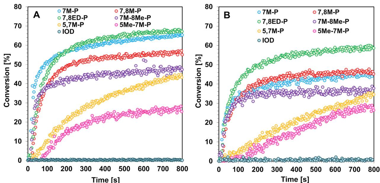
Fig. 5 Photopolymerization profiles of a 25  $\mu\text{m}$  thick coating consisting of the CADE monomer and studied coumarin iodonium salts under (A) LED@365 nm and (B) LED@405 nm exposure.
