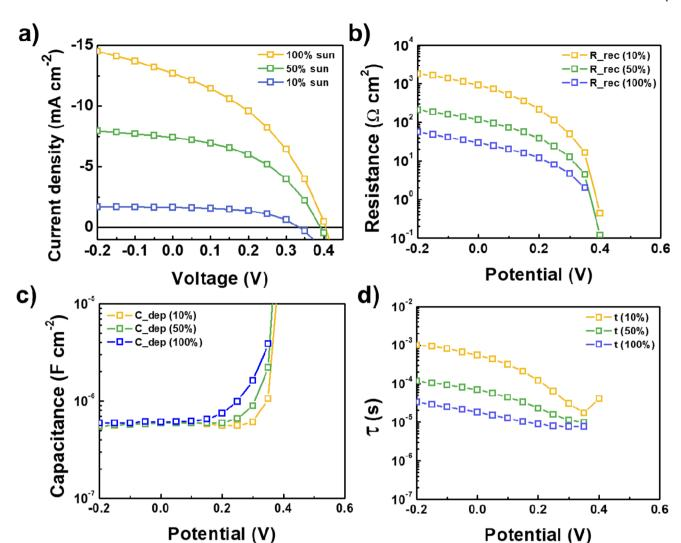
Fig. 3 (a) Steady-state photocurrent densities obtained by the w-seed Sb<sub>2</sub>Se<sub>3</sub> PV during IS measurement under 10%, 50%, and 100% sun illumination. (b) Resistances (c) capacitance, and (d) time constants for charge transfer of the w-seed Sb<sub>2</sub>Se<sub>3</sub> PV from the IS fitting procedure.
