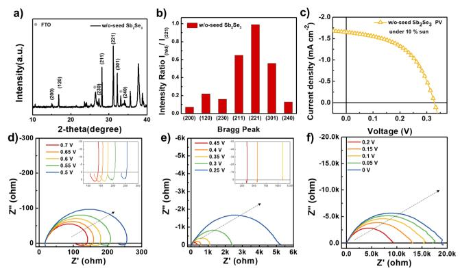
Fig. 4 (a) Diffraction patterns and (b) peak intensities ratio  $(l_{(hkl)}/l_{(221)})$  of the obtained w/o-seed Sb<sub>2</sub>Se<sub>3</sub> films (c) J-V behavior exhibited by the w/o-seed Sb<sub>2</sub>Se<sub>3</sub> PV under 10% sun illumination. (d-f) Nyquist plots of the w/o-seed Sb<sub>2</sub>Se<sub>3</sub> PV at the designated applied potential.
