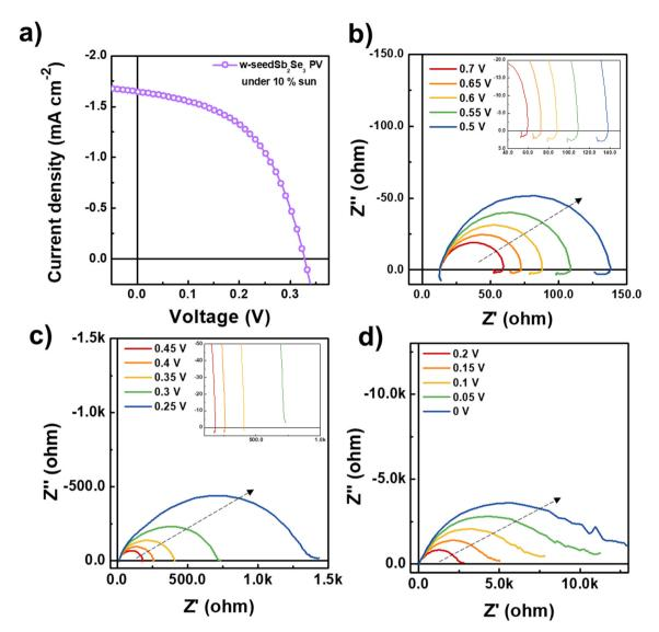
Fig. 2 (a) J-V curve of the w-seed Sb<sub>2</sub>Se<sub>3</sub> PV under 10% sun illumination. (b-d) Nyquist plots of the w-seed Sb<sub>2</sub>Se<sub>3</sub> PV at the designated applied potential.
