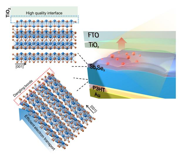
Fig. 6 Schematic illustration of the proposed novel bilayer Sb<sub>2</sub>Se<sub>3</sub> configuration that can effectively transport the charge carriers without recombination and also form a high quality interface with the TiO<sub>2</sub> layer.
