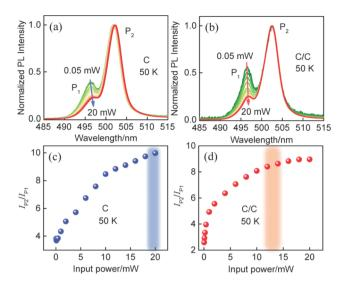
Fig. 3 Power-dependent PL spectra of (a) C and (b) C/C NPLs at 50 K. (c) C and (d) C/C NPLs Power-dependent ratio of  $P_2/P_1$ . The cylinders represent the initial saturation power of C and C/C NPLs, respectively.
