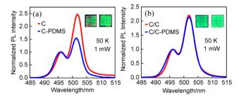
Fig. 4 Normalized PL spectra of the samples before and after PDMS treatment (a) C and (b) C/C NPLs at 50 K. Inset: images of the samples before and after PDMS treatment under UV light illumination.
