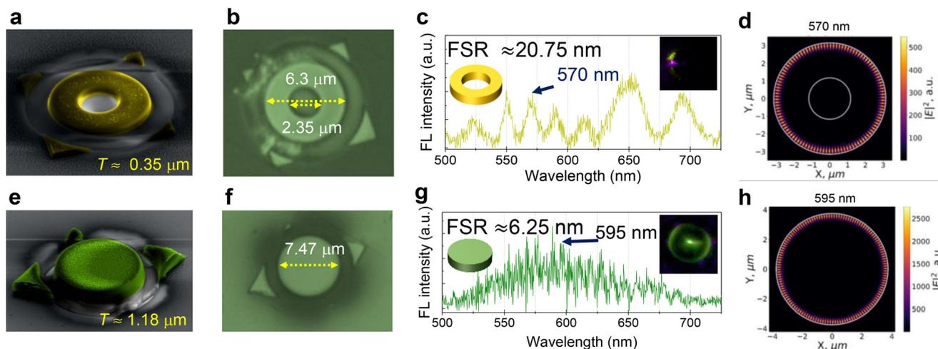
**Fig. 3** (a and e) The color-coded FESEM images, (b and f) optical microscopy images and (c and g) the corresponding FL background subtracted spectra of the fabricated perylene and coumarin-153 microresonators, respectively. The insets in (c) and (g) show the FL images during focused optical excitation. FDTD calculations displaying (d)  $|E|^2$  distribution for the 570 nm mode in the ring resonator and (h) 595 nm mode in the disc resonator.
