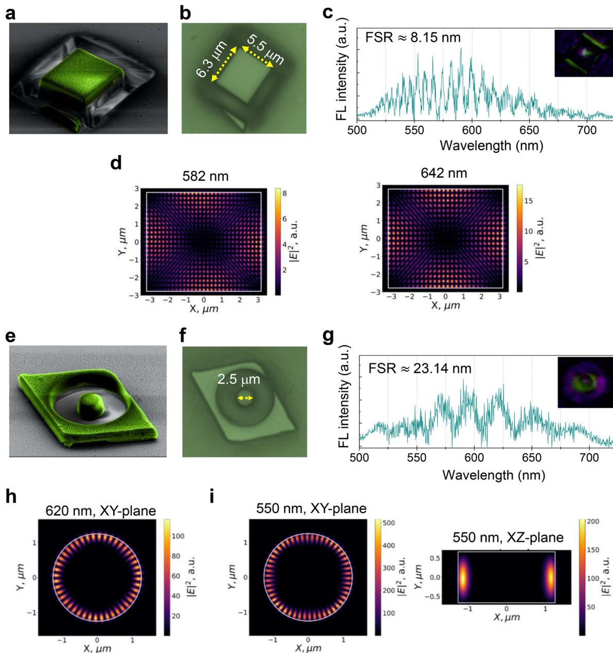
**Fig. 4** (a and e) Colored FESEM images, (b and f) optical microscopy images, and (c and g) the corresponding FL background-subtracted spectra of microrectangle and microdisc of coumarin-153, respectively. Insets in (c) and (g) show the corresponding FL image. FDTD calculations displaying  $|E|^2$  distribution for (d) 582 nm and 642 nm modes for the rectangular-shaped resonator and (h and i) 620 nm and 550 nm microdisc of coumarin-153.
