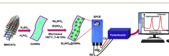
Fig. 12 Schematic illustration for the preparation of Bi 2 WO 6 @GNRs nanocomposite for sensing dihydroxybenzene isomers in water samples and face cream sample. WE = working electrode, RE = reference electrode, CE = counter electrode (reprinted from ref. 157 with permission from Elsevier Publisher).
