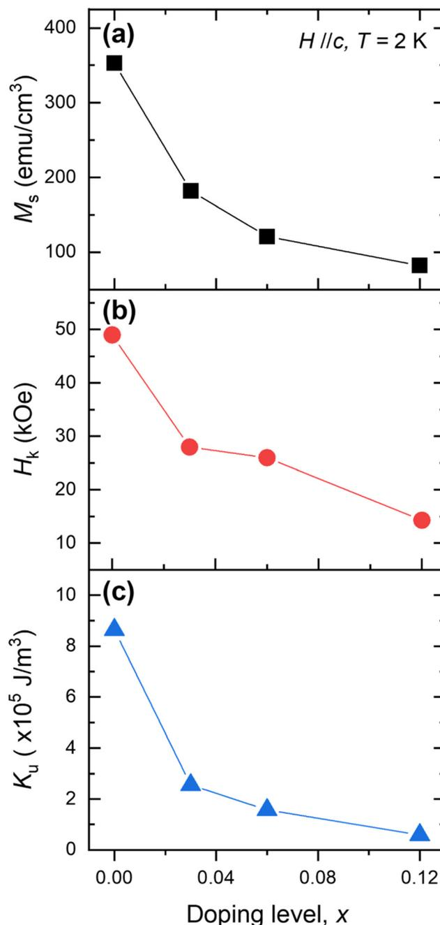
Fig. 5 Doping level dependence of the FM characteristics of FNGT. (a)  $x$  dependence of the saturation magnetization ( $M_s$ ) of FNGT. (b)  $x$  dependence of the anisotropy field ( $H_k$ ) of FNGT. (c)  $x$  dependence of the anisotropy energy ( $K_u$ ) of FNGT. All data are measured with  $H//c$  at 2 K.
