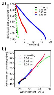
Fig. 2 . (a) Kinetics of the reflection peak wavelength as a function of shellac layer thickness upon drying. (b) Reflection peak wavelength as a function of HPC/water ratio for samples with different shellac coating thicknesses. The colours shown in the graphs represent different thicknesses of the shellac layer: no coating (black), 2.08 um-thickness (green), 3.56 um-thickness (red), and 5.46 um-thickness (blue)
