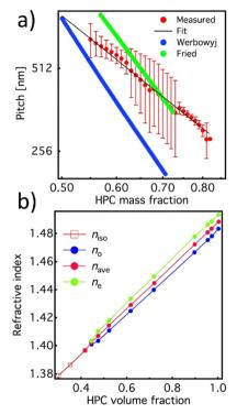
Fig. 3 (a) Extrapolated cholesteric pitch values (red line: experiment and black line: fit) as a function of the HPC/water ratio acquired with the balance and compared with the literature values from Werbowyj<sup>5</sup> (blue line) and Fried<sup>20</sup> (green line). (b) Value of the average refractive index (red) of the HPC mesophase extrapolated from ordinary and extraordinary values of refractive index calculated using eqn (1).
