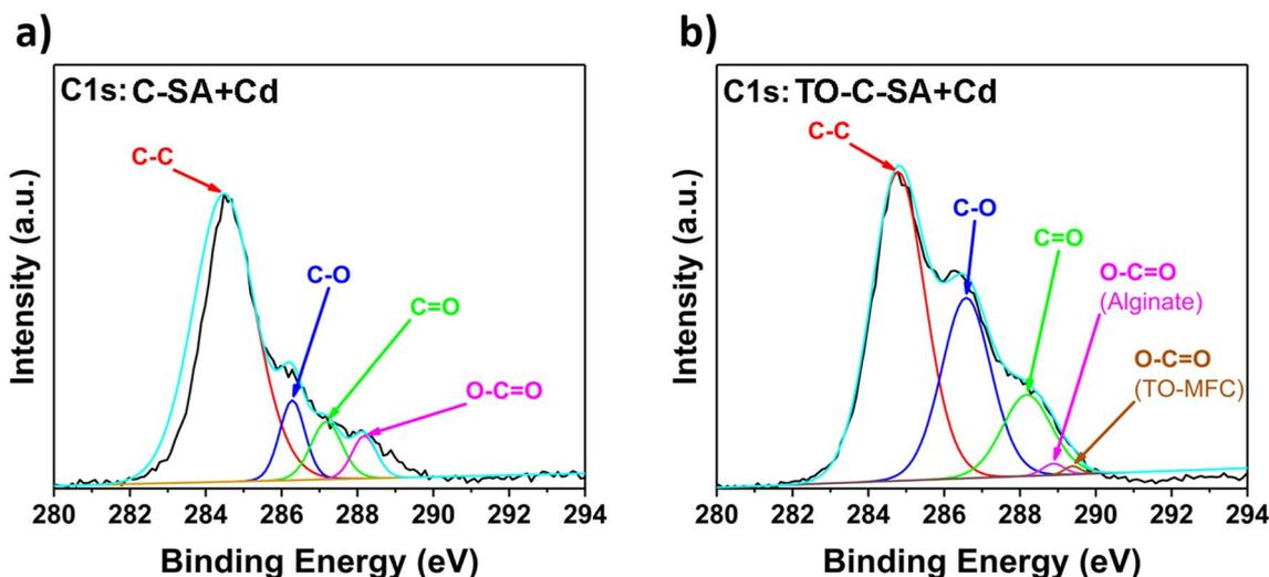
Fig. 6 C 1s high-resolution XPS spectra of (a) C-SA and (b) TO-C-SA beads after Cd<sup>2+</sup> adsorption.
