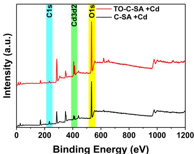
Fig. 5 XPS survey of C-SA and TO-C-SA beads after Cd<sup>2+</sup> adsorption.
