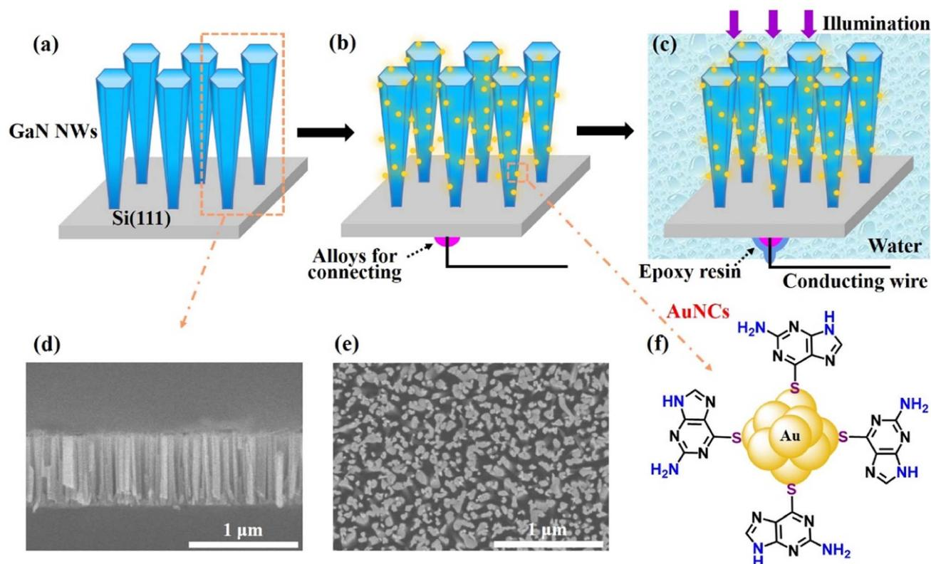
**Fig. 1** (a) Grow the GaN NWs on the Si substrate using MBE. (b) Coat the AuNCs onto the NW surfaces and connect the conducting wire. (c) Measure the PD under illumination. (d) Side-view and (e) top-view scanning electron microscopy (SEM) images of GaN NWs. (f) Schematic structure of AuNC crystals.
