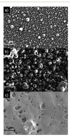
Fig. 5 SEM images of PPy grown to a charge density of 210 mC cm $^{-2}$  onto (a) Au and (b) PSI/Au. A drop-cast film of PSI (no Ppy) is shown in (c) as a comparison.
