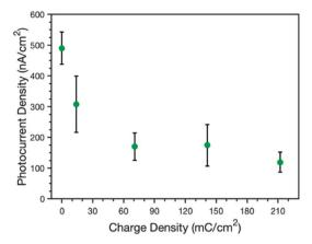
Fig. 7 Effect of charge density of electrodeposited PPy on the peak photocurrent density of PSI/Au films. Measurements were made in 0.1 M KCl (ag) containing AscH/DCPIP (20:1 mM) as redox mediators. All films were illuminated for 30 s and the peak current typically occurred within the first 2 s.
