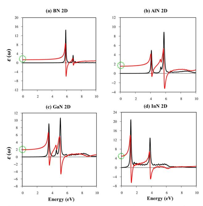
Fig. 9 (a-d) The real part and imaginary part of the dielectric functions with exciton effects (red and black curves, respectively) of the BN, AlN, GaN, and InN monolayers, respectively. The dashed green circles correspond to dielectric constants.
