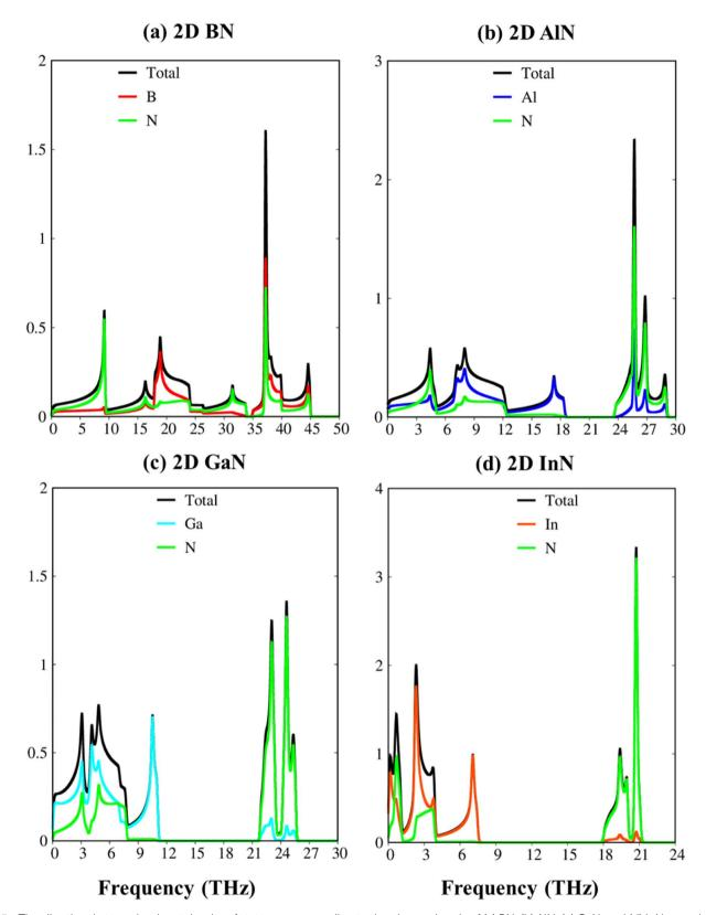
Fig. 3 The vibrational atom-dominant density of states, corresponding to the phonon bands of (a) BN, (b) AlN, (c) GaN, and (d) InN monolayers.
