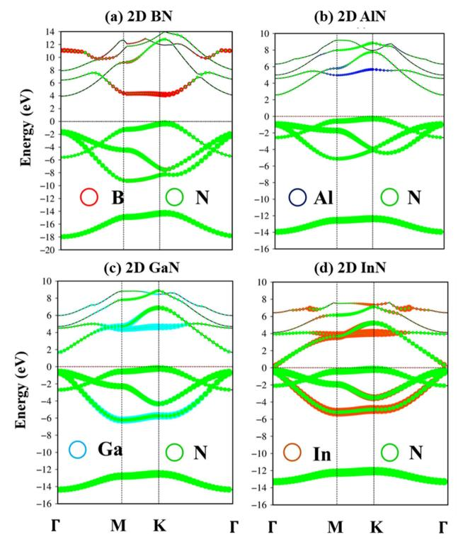
Fig. 5 (a-d) B, Al, Ga, In, and N atoms of BN, AlN, GaN, and InN two-dimensional monolayers are represented by red, blue, cyan, orange, and green balls, respectively.
