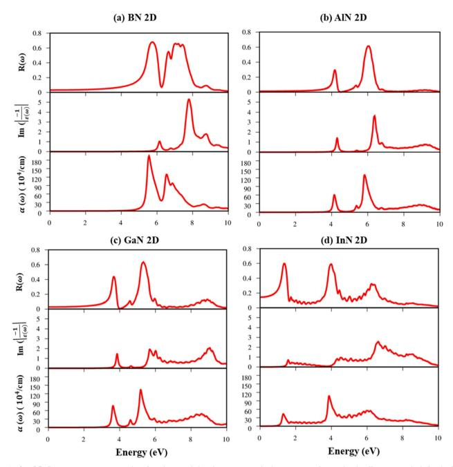
Fig. 10 (a-d) Reflectance spectra, energy loss functions, and absorbance spectra in the presence of an excitonic effect, respectively for the BN, AIN, GaN, and InN monolayers.
