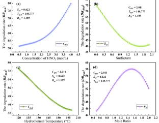
Fig. 9 SA of the four features based on the SVR-RBF model (a)  $C_{HN}$ , (b)  $S_{\rm ur}$ , (c)  $T_{\rm hyd}$  and (d)  $R_{\rm m}$ .
