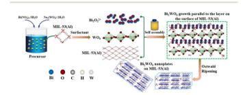
Fig. 3 The formation mechanism of BWO/MIL.
