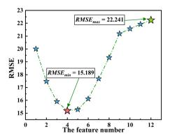
Fig. 4 The process of feature selection in FFS-SVR.
