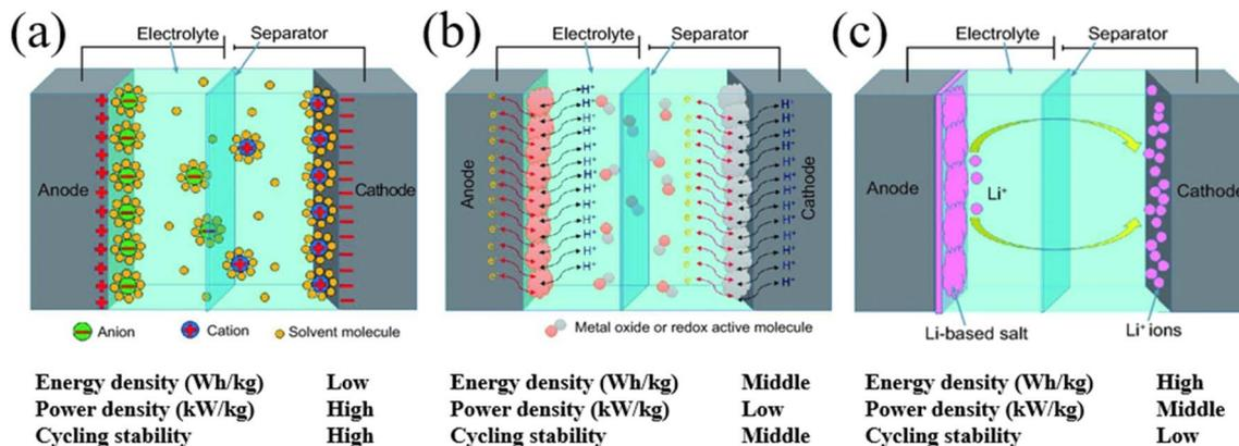
Fig. 2 Schematic of (a) an electrical double-layer capacitor (EDLC), (b) a pseudocapacitor, and (c) a hybrid supercapacitor.<sup>10</sup> [This figure has been adapted/reproduced from ref. 10 with permission from OXFORD UNIVERSITY PRESS, copyright 2017.]
