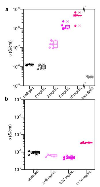
Fig. 1 Conductivity as a function of doping with (a) Sml2 and (b) Sml3.  $0~{
