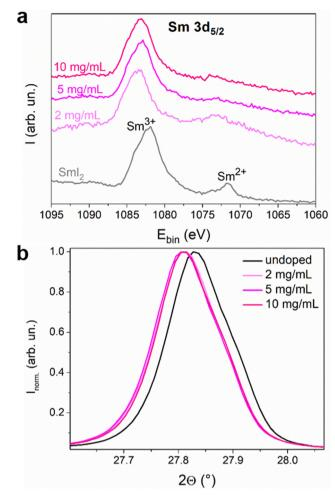
Fig. 2 (a) XPS spectra of a thin film of  $Sml_2$  and perovskite thin films with different doping concentrations. The spectra are separated on the Y-axis for clarity. (b) Normalized X-ray diffraction (200) peaks of undoped and doped MAPI films.
