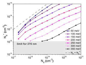
Fig. 9 Impact of the dopant energy level  $E_{\rm d}$  on the ionized dopant concentration extracted from the simulated  $1/C^2$  plot *versus* the real dopant concentration.  $E_{\rm d}$  is varying from 50 meV to 350 meV to highlight the effect of the dopant energy level  $E_{\rm d}$  on the charge carrier density.  $E_{\rm d}$  = 350 meV has been determined with conductivity *versus* temperature measurements.
