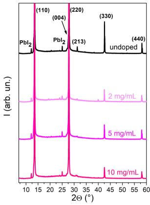
Fig. 4 XRD spectra of the undoped MAPI film and MAPI doped with concentrations of 2-20 mg mL<sup>-1</sup>. For higher doping concentrations, see Fig. S9 (ESI†).
