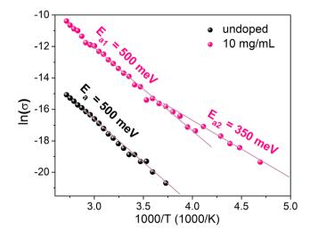
Fig. 8 Temperature dependent conductivity of the undoped MAPI film and MAPI doped with 10 mg mL<sup>-1</sup> Sml<sub>2</sub>.
