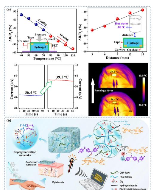
Fig. 11 (a) A temperature sensor serves to monitor a human forehead's temperature. Reprinted from ref. 22 with permission. Copyright 2020 American Chemical Society. (b) The design of a PANI based hydrogel with strain and temperature responsiveness. Reprinted from ref. 242 with permission. Copyright 2022 Elsevier.
