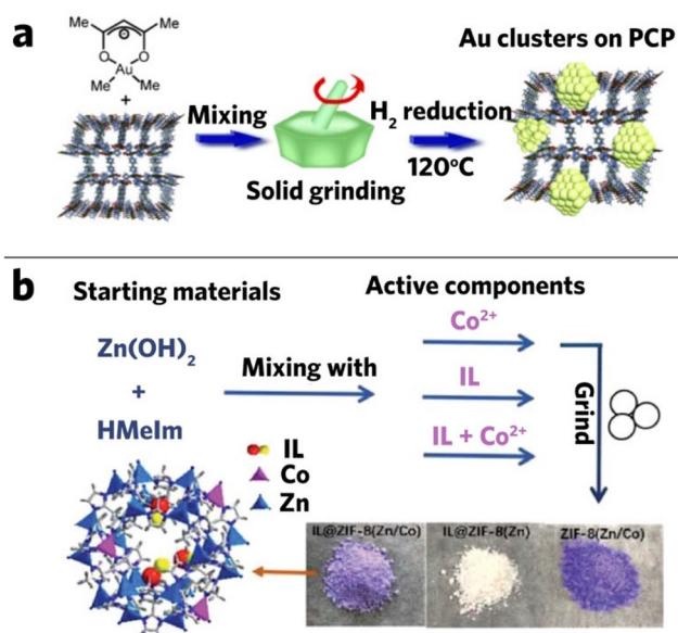
Fig. 10 (a) Mechanochemical deposition of gold clusters on porous coordination polymers. Reproduced with permission from ref. 100, (b) synthetic procedures of L@ZIF-8(Zn/Co). Reproduced with permission from ref. 133.
