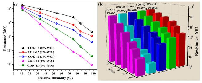
Fig. 9 (a) Humidity response curves; (b) 3-D bar chart, illustrating resistance reduction with increasing %RH for COK-12 and WO<sub>3</sub>/COK-12 nanostructures
