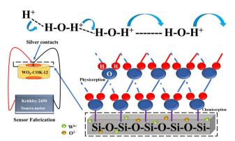
Fig. 12 Illustration of the Grotthuss chain mechanism in WO<sub>3</sub>/COK-12 showcasing the proton-conducting process within the sensing material.
