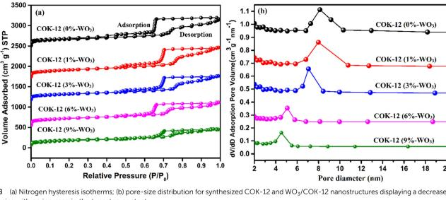
Fig. 8 (a) Nitrogen hysteresis isotherms; (b) pore-size distribution for synthesized COK-12 and WO<sub>3</sub>/COK-12 nanostructures displaying a decrease in the pore size with an increase in the tungsten content.
