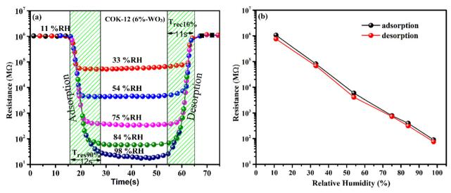
Fig. 10 (a) Response/recovery curve across diverse humidity levels for the 6%-WO3/COK-12 configuration; (b) Hysteresis curve displaying the lag between the adsorption and desorption process of the sensor
