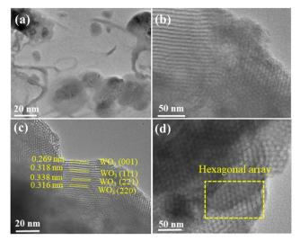
Fig. 6 HRTEM micrographs illustrating uniform pore channels: (a) and (b) COK-12 and (c) and (d) 6%-WO<sub>3</sub>/COK-12 at 20 and 50 nm, respectively.
