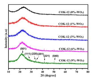
Fig. 3 WAXRD profiles revealing the crystalline structure of COK-12 and  $WO_{\pi}/COK$ -12 nanostructures.
