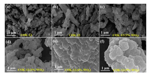
Fig. 4 FESEM recorded micrographs illustrating a granule-type morphological structure: (a) and (b) COK-12 and (c)-(f) WO<sub>3</sub>/COK-12 nanostructures.
