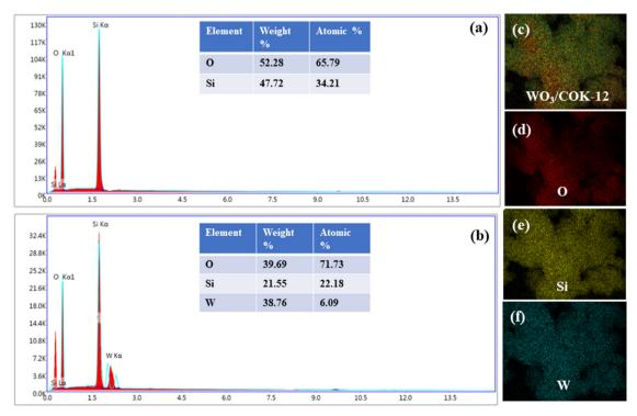
Fig. 5 EDX analysis describing the elemental composition: (a) COK-12 and (b) 6%-WO<sub>3</sub>/COK-12 and (c)-(f) EDX elemental mapping
