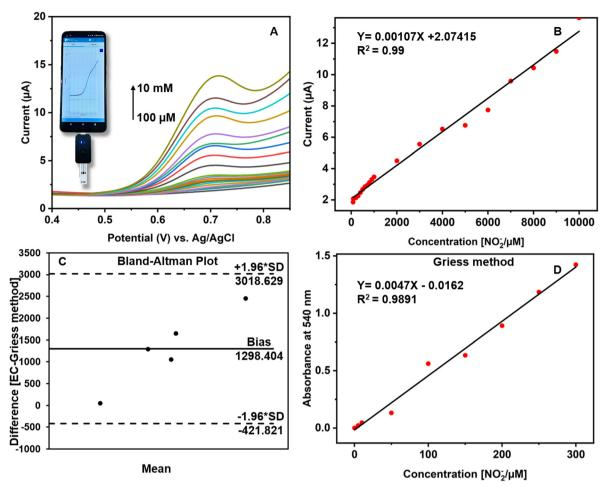
Fig. 5 (A) LSV response of the CuCP-MWCNTs-SPCE towards various concentrations of nitrite ranging from 100 μM to 10 mM. Calibration plot of the CuCP-MWCNTs-SPCE towards nitrite detection in human saliva samples (B). Comparison of the electrochemical and Griess method results using a Bland-Altman plot (C). Calibration plot of the Griess method towards nitrite detection in human saliva samples (D).
