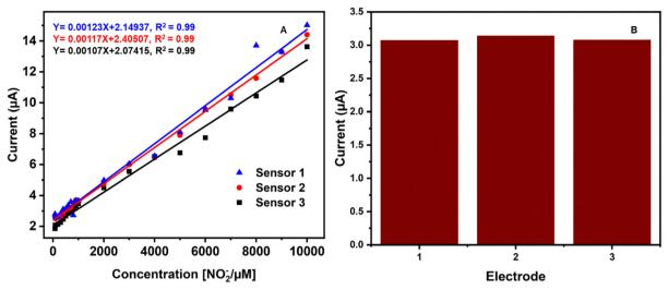
Fig. 6 Reproducibility investigation of CuCP-MWCNTs-SPCE towards nitrite detection with the (a) calibration curves for the concentration between 100 μM and 10 mM; (b) intra-study of three sensors in 500 μM nitrite in saliva samples with 0.01 M PBS.
