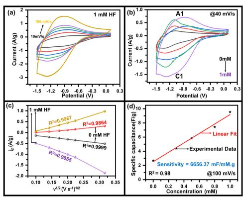
Fig. 2 CV graph of  $MoO_3$  at GCE with (a) 1 mM HF, (b) 0 mM, 0.2 mM, 0.5 mM, 0.8 mM, and 1.0 mM HF in 0.5 M LiClO<sub>4</sub> in PC, (c) variation of current density ( $j_0$ ) vs.  $v^{1/2}$  graph with and without HF, and (d) variation of specific capacitance with concentration of HF including raw data and linear fit.
