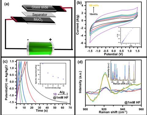
Fig. 4 (a) Schematic diagram of as-fabricated MoO<sub>3</sub>//AC supercapacitor device, (b) CV curves measured at scan rates of 10 to 100 mV s<sup>-1</sup> along with the corresponding EIS plot (ESI†), (c) GCD plots at 2 A g<sup>-1</sup> to 10 A g<sup>-1</sup> along with variation of specific capacitance as a function of current density (inset) and (d) in situ Raman spectra of asymmetric supercapacitor device during the charging and discharging process.
