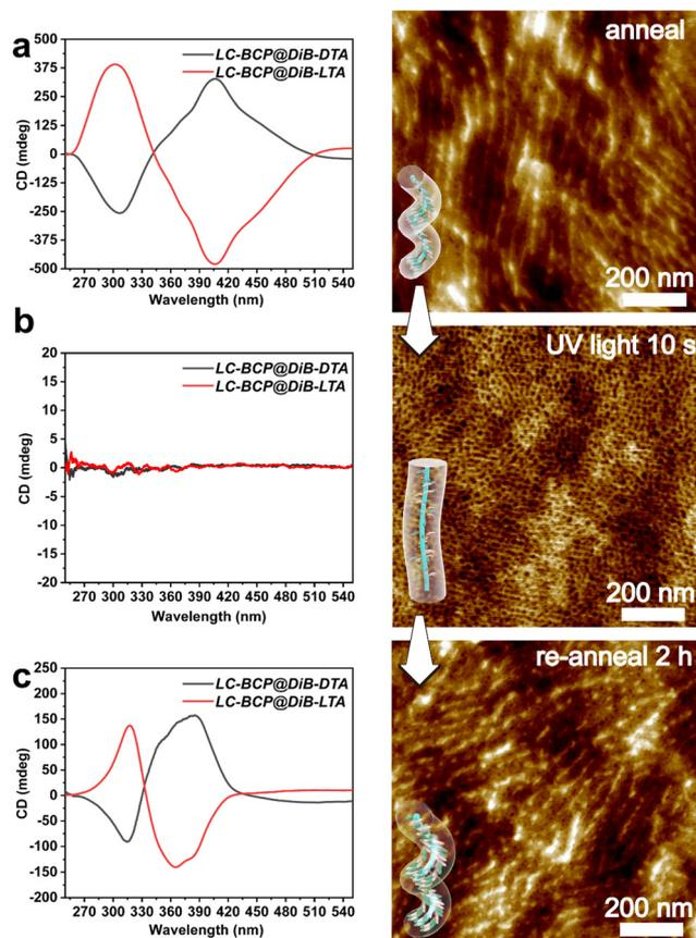
**Fig. 6** CD spectra and AFM image of LC-BCP@DiB-LTA film before (a) and after (b) UV irradiation (10 s, 365 nm, 150 mW cm<sup>-2</sup>), and the recovered helical structure after re-annealing for 2 h (c).
