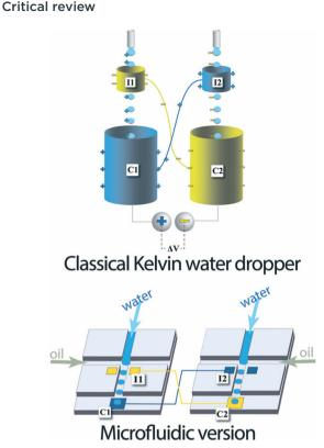
Fig. 1 Top, classical Kelvin water dropper, bottom, representation of the microfluidic version (figures and captions reproduced from ref. 16 with permission from Royal Society of Chemistry, copyright 2013).
