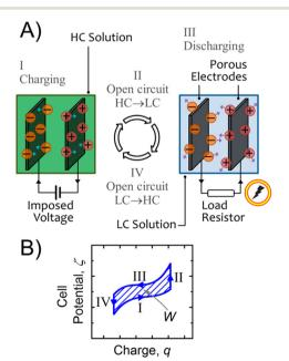
Fig. 20 (A) Illustration of the working principle of capacitive energy extraction based on double layer expansion (CDLE) and (B) the qualitative plot of useful work W produced in an unit Capmixing cycle (figures and captions reproduced from ref. 69 with permission from American Chemical Society, copyright 2016).
