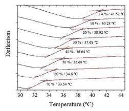
Fig. 3  $T_{\rm q}$  variation (from 42 °C to 34 °C) as a function of humidity in the range between 1.4% and 70%. Reprinted with permission from reference Polym. Test., 2018, 65, 407-413. 112 Copyright 2018 Elsevier.
