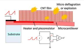
Fig. 7 Schematic illustration of the sensor configuration and the operation principle vapors adsorbed on the CNT sensor after heating to micro deflagration. Reprinted with permission from ref. 179. Copyright 2013 Elsevier.
