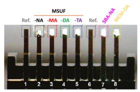
8 Optical microscopy image of the sorbent-coated microcantilever array. Reprinted (adapted) with permission from reference Environ. Sci. Technol., 2011, 45(13), 5704-5709. 192 Copyright 2011 American Chemical Society.
