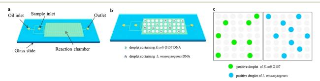
Fig. 10 Droplet digital PCR workflow for simultaneous detection of E. coli O157 and L. monocytogenes. (a) Fabrication of mineral oil saturated PDMS (OSP) microfluidic chip. (b) Generation of droplets. (c) On-chip amplification under many times of thermal cycles followed by fluorescence readout. Copyright 2015 by Elsevier. 126
