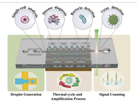
Fig. 1 Schematic diagram of ddPCR and applications.
