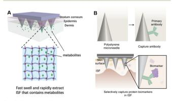
Fig. 2 Schematic illustrations of different extraction mechanisms of (A) swelling-based extraction. Reproduced with permission.<sup>51</sup> Copyright 2017, Wiley-VCH Verlag. (B) Antibody-based extraction. Reproduced with permission.<sup>56</sup> Copyright 2021, Springer Nature
