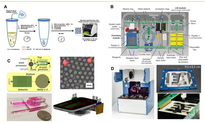
Fig. 6 Approaches to integrating the assay and single molecule detection steps in DBA. A) Manual pipetting of reagents and automated washing (ref. 90). B) Fully automated system for assays and imaging (ref. 50). C) Miniaturized assay processing based on pressure-driven microfluidics and flow detection on a mobile phone of beads in water-in-oil droplets (ref. 59). D) Miniaturized assay processing based on DMF (ref. 81). Figures reproduced with permissions.
