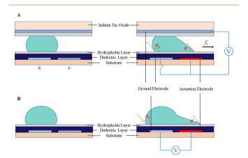
Fig. 3 Schematic diagram of droplet actuation in A) two parallel plates and B) single plate due to the asymmetric contact angle across the droplet.
