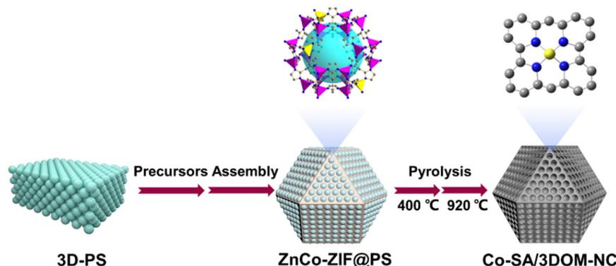
Fig. 1 Schematic illustration of the fabrication of Co-SA/3DOM-NC.
