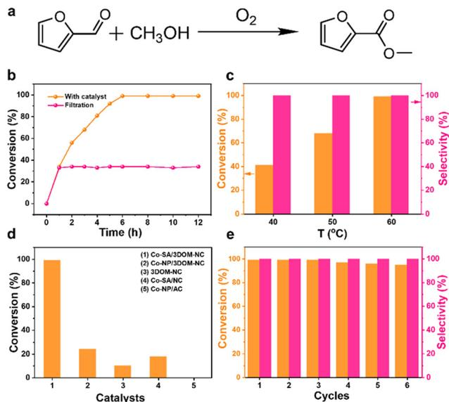
**Fig. 6** (a) Catalytic oxidative esterification of FFA to methyl 2-furoate. (b) Activity profiles for the oxidation esterification of FFA over Co-SA/3DOM-NC. (c) The effects of temperature on the FFA conversion and methyl 2-furoate selectivity over Co-SA/3DOM-NC. (d) The comparison of the FFA conversion between Co-SA/3DOM-NC and other catalysts. (e) Reusability tests of Co-SA/3DOM-NC for the oxidative esterification of FFA.
