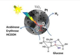
Fig. 8 Graphical illustration of the photoconversion of Glc in the presence of Pt-loaded  $TiO_2$  catalysts. Reproduced with permission from ref. 94. Copyright 2016, Elsevier.
