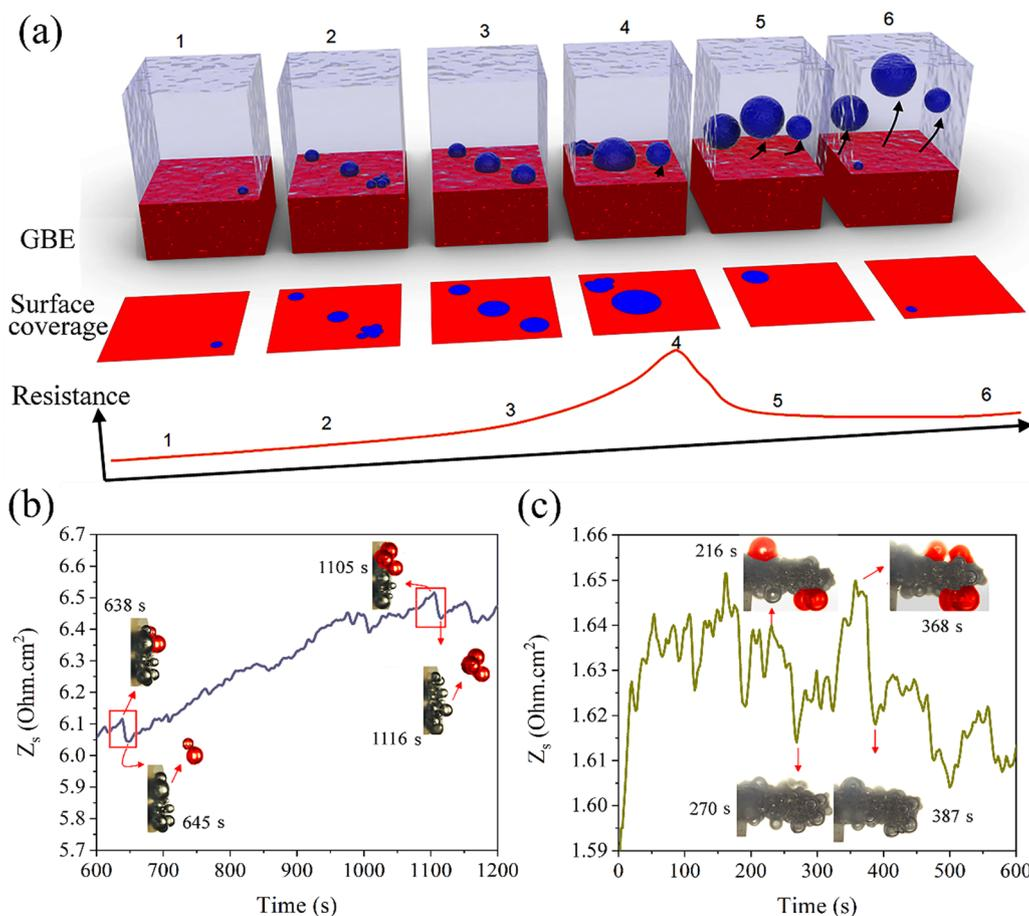
**Fig. 1** (a) Schematic representation of dynamic resistance variation *via* single frequency impedance. *Operando* dynamic resistance variation at 10 kHz for the HER in 1 M KOH with the corresponding GBE captured at selected time intervals on (b) the GCE at  $-1.45$  V and (c) the NF at  $-0.15$  V (V vs. RHE).
