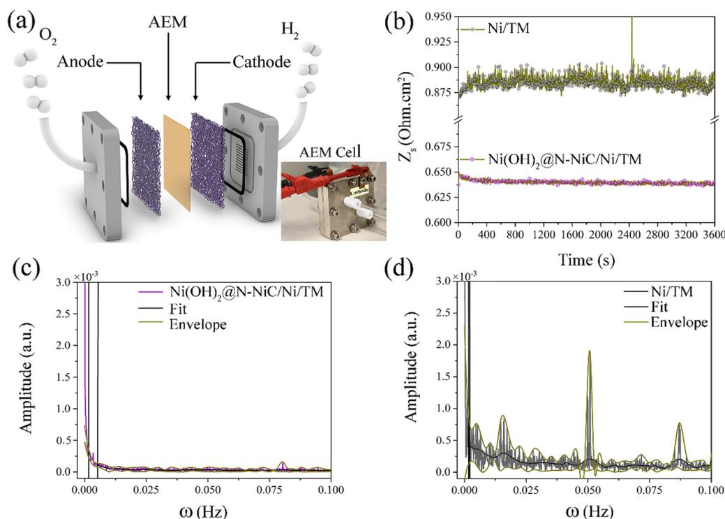
Fig. 4 (a) Schematic representation and photograph of an AEM water electrolyser. (b) Dynamic resistance variation at 10 kHz and 500 mA cm<sup>-2</sup> and the corresponding FFT plots of (c) Ni(OH)<sub>2</sub>@N-NiC/Ni/TM, and (d) Ni/TM, each used as both anode and cathode.
