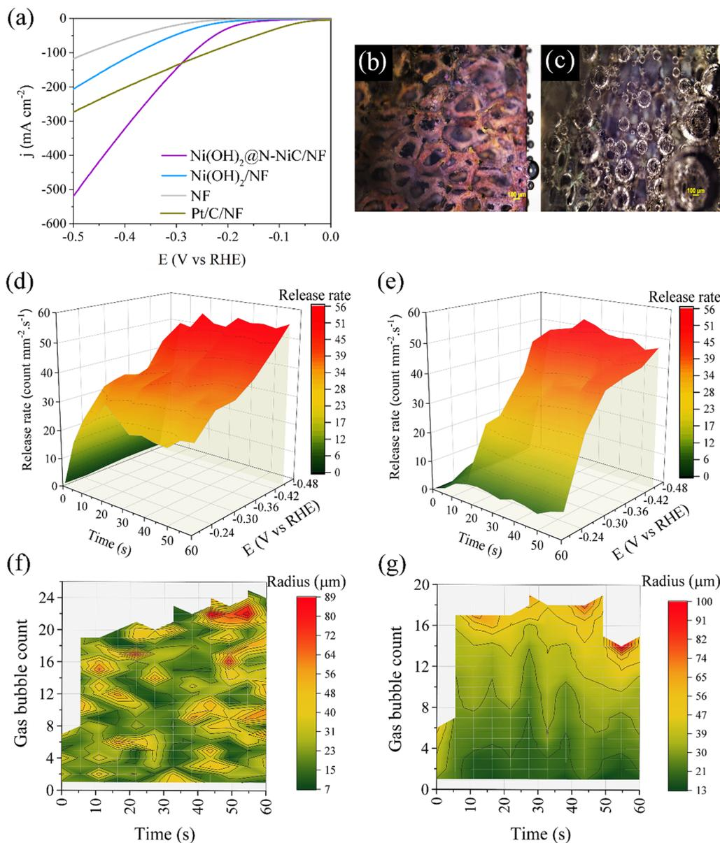
Fig. 2 (a) HER polarization curves. Optical images of gas bubbles over (b) Ni(OH)<sub>2</sub>@N-NiC/NF and (c) Ni(OH)<sub>2</sub>/NF at 0.245 V vs. RHE. *Operando* optical microscopy: 3D surface plots of (d) Ni(OH)<sub>2</sub>@N-NiC/NF and (e) Ni(OH)<sub>2</sub>/NF. Contour plots at 0.445 V vs. RHE for (f) Ni(OH)<sub>2</sub>@N-NiC/NF and (g) Ni(OH)<sub>2</sub>/NF.
