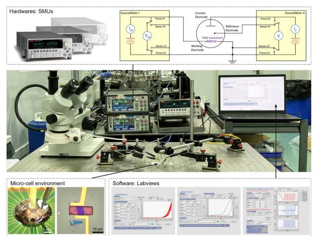
Fig. 5 The typical testing setups used in our lab. The hardwares involved in the test are source measurement units (SMUs), and the software is Labview. Taking in situ electronic/electrochemical measurement as an example, SMU 1 and SMU 2 are used for the electronic and the three-electrode electrochemical measurements, respectively, as the equivalent circuit diagram shows
