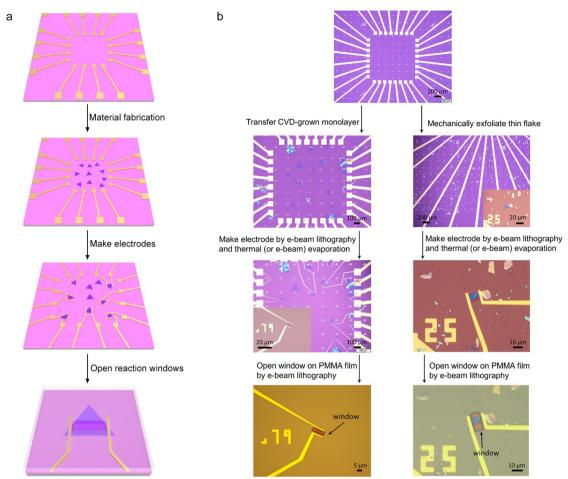
Fig. 4 Fabrication process of an on-chip microcell. (a) Schematic illustration of the fabrication steps of the on-chip microcell. (b) Typical fabrication procedures in 2D TMD-based microcells, in which CVD-grown and mechanically-exfoliated samples were introduced, respectively.
