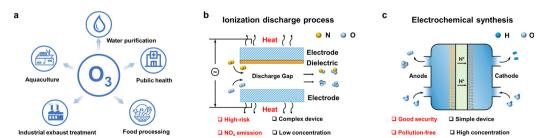
Scheme 1 Applications and preparation methods of ozone. (a) Applications of ozone in various industries. (b) Ozone preparation through the ionization discharge process. (c) Ozone preparation by the electrochemical oxidation of water.
