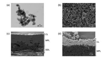
Fig. 1 (a) Representative TEM image of the synthesized CuONPs. (b) Topview and (c and d) cross-sectional SEM micrographs of CuONPs-1.7/GDE.
