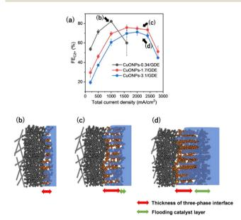
Fig. 4 (a)  ${\rm FE_{C_{2+}}}$  against  $J_{\rm total}$  for various amounts of Cu loading (CuONPs-0.34, -1.7 and -3.1/GDE) in 1 M KCl. (b-d) Schematic image of the threephase interfaces at each position which are indicated in (a). The red and green arrows represent the thickness of three-phase interface and flooding catalyst layer, respectively
