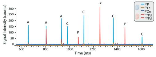
Fig. 3 The time trace of THP-1 cells exposed to 5  $\mu q$  L<sup>-1</sup> Pd-doped nanoplastics where different species can be recognized as pulses above the background. Namely: (C) single THP-1 cells without associated nanoplastics, (P) nanoplastics and (A) associated events.
