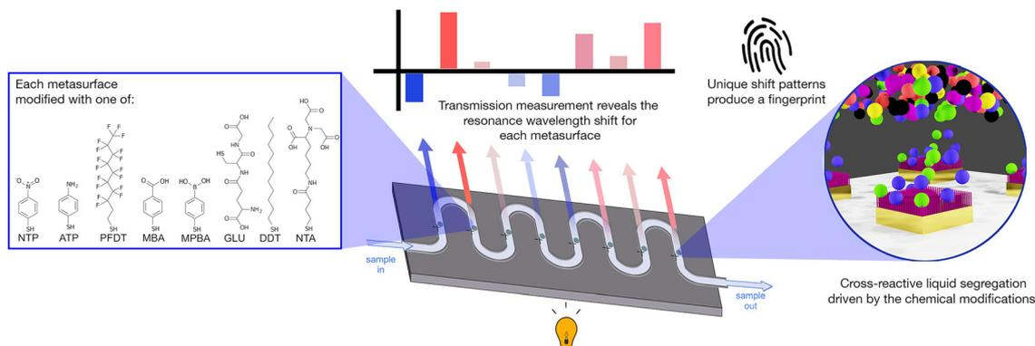
**Fig. 1** Schematic of the sensor concept. Eight metasurfaces are linked by a microfluidic channel. Each metasurface is modified with a different surface chemistry, providing partial-selectivity to the components in the water sample. Thus, each metasurface experiences a unique refractive-index environment, shifting its resonance wavelength value. By tracking the combination of resonance shifts we build a fingerprint for each sample.
