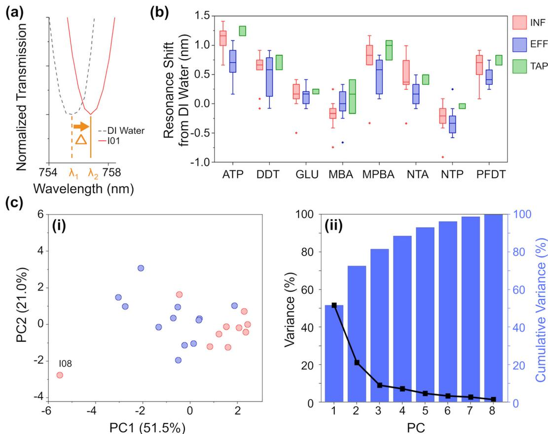
**Fig. 3** (a) Example of a resonance redshift from DI water (ATP chemistry, sample I01). (b) Resonance shift from DI water of each NTB grouped by water sample type. (c) PCA of the resonance shift (average shift from DI water) for INF and EFF: (i) scatterplot of the first and second principal components and (ii) a plot of the variance and cumulative variance as explained by each PC.
