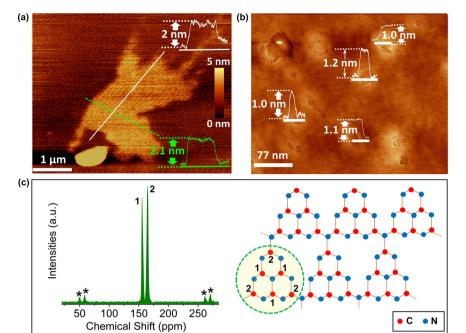
Fig. 2 (a) AFM image of q-CN nanosheet with sectional profile measurement showing height and thickness profiles (nm). (b) AFM images of nanosheets with respective height profiles at different locations. (c) Solid-state <sup>13</sup>C NMR spectra of as-prepared g-CN and its idealized structure showing heptazine tectonic units
